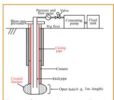
Figure 1. Schematic borehole configuration during a leak-off test (LOT) or extended leak-off test (XLOT; after Yamamoto, 2003)
