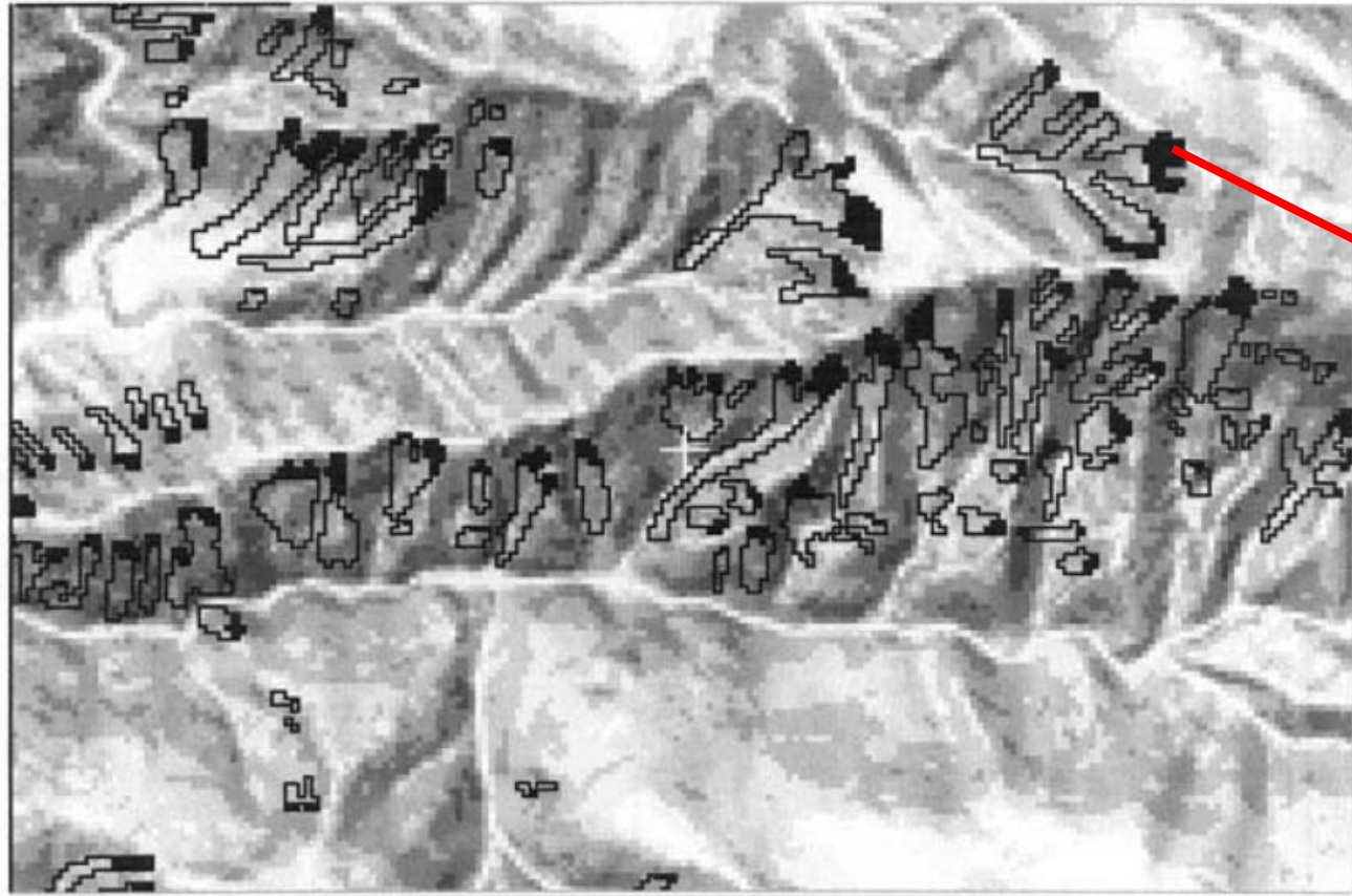
Scars of the past landslides induced by the 1994 Northridge Earthquake in California, U.S.A.
