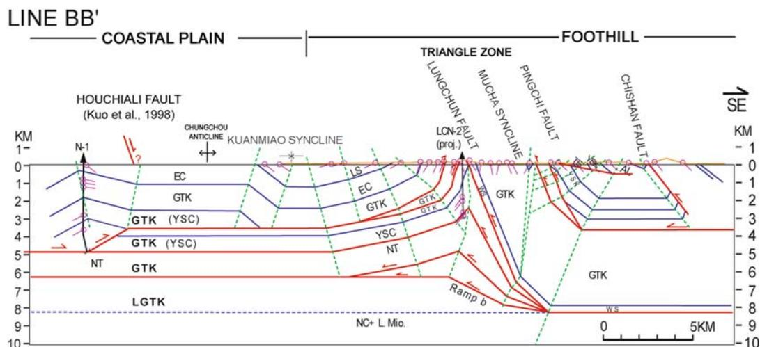
Figure 7. Line BB' illustrating changes in structural style from east to west. Location of Line BB' is shown on Figure 2. Line BB' illustrates the triangle zone wedge signature moving westward.
