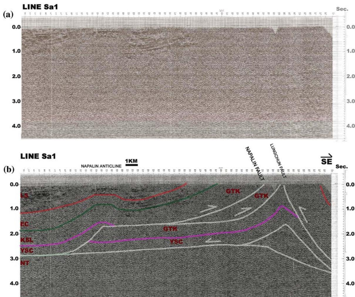
Figure 5. Seismic section Sa1 illustrating the geometry of Napalin anticline (see Figure 1 for location). Line Sa1 illustrates seismic signature of Napalin anticline with a gentle west limb and steep east limb. (a) uninterpreted seismic section Sa1, (b) Interpreted seismic section showing the Napalin anticline is formed by back-thrusting. Structures underneath the Lungchuan Fault include triangle underlying by thrust imbrication.
