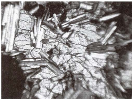
Figure 3–8 Ophitic texture. A single pyroxene envelops several well-developed plagioclase laths. Width 1 mm.
