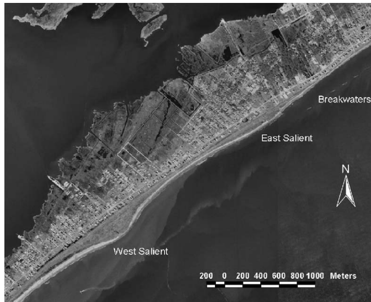
Fig. 2. Aerial photograph showing salients shoreward of borrow area along Grand Isle, LA in 1998 (modified from Louisiana Oil Spill Coordinator's Office (LOSCO), 1999).
