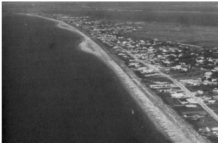
Fig. 1. Aerial photograph showing salients shoreward of borrow area looking East to West along Grand Isle, LA in August, 1985 (Combe and Soileau, 1987).
