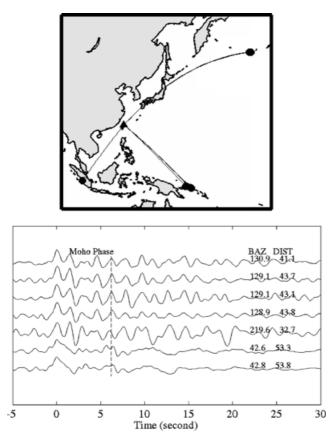
**Figure 14.** (a) Examples of radial-component receiver functions for NACB station north of the suture zone between the Philippine Sea and the Eurasian plates showing similar receiver function waveforms for earthquakes from all directions except the northeast direction. (b) Inversion results for NACB station are shown with the same format as in Fig. 7. The preferred Moho depth is around 50–52 km.
