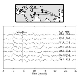
Figure 11. (a) Examples of radial-component receiver functions for TPUB station in southwestern Taiwan showing similar receiver function waveforms for earthquakes from the west. (b) Inversion results for TPUB station are shown with the same format as in Fig. 7. A mid-crust discontinuity can be identified at depth  $\sim$ 20 which can be interpreted as the Conrad discontinuity. The preferred Moho depth is around 30–32 km.
