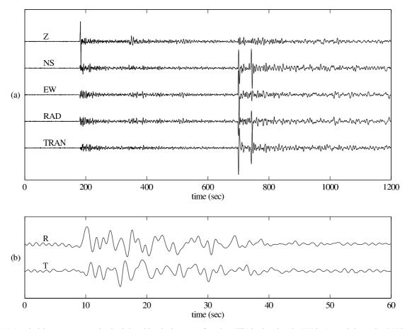
Figure 4. (a) A typical three-component teleseismic broad-band seismogram for a deep Fiji Island earthquake (573 km) recorded at station TATO (upper three traces); and the radial and transverse components after rotation (fourth and fifth traces). (b) Radial (R) and transverse (T) receiver responses after a source equalization (deconvolution) process.
