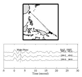
**Figure 9.** (a) Examples of radial-component receiver functions for TWB1 station in the northeastern corner of Taiwan showing similar receiver function waveforms for earthquakes from the southeast. (b) Inversion results for TWB1 station are shown with the same format as in Fig. 7. The preferred Moho depth is around 20–30 km.
