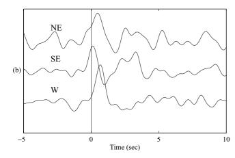
Figure 18. (a) Radial-component receiver functions for ANPB station, where receiver functions can be grouped into three groups according to their backazimuths and waveform similarities. (b) Stacked receiver functions for the NE, SE, and W groups show different onset times (although the background is relatively noisy). The onset time delay can be as large as 0.7 s along the W direction, which may suggest a west-dipping structure just beneath the free-surface.
