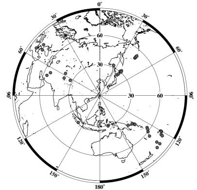
Figure 3. Map showing epicentres of the selected teleseismic events (solid circles) used in this study. Earthquakes are selected based on consideration of epicentral distance ( $25^{\circ} < \Delta < 100^{\circ}$ ), magnitude (>6.5), and high signal-to-noise ratio on observed seismograms.
