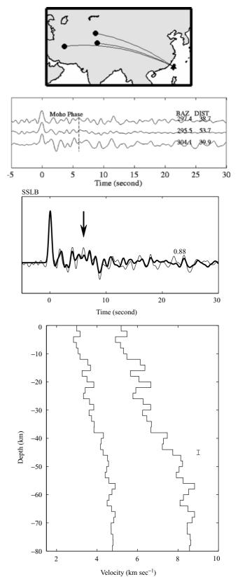
**Figure 12.** (a) Examples of radial-component receiver functions for SSLB station in the Central Mountain Range showing similar receiver function waveforms for earthquakes from the western direction. (b) Inversion results for SSLB station are shown with the same format as in Fig. 7. Crustal velocities increase steadily as a function of depth from the surface to the bottom of the crust. The preferred Moho depth is around 44–46 km.
