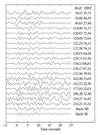
**Figure 16.** Examples of transverse-component receiver functions recorded at TATO station. Tangential receiver functions for the first three events from similar azimuths are stacked to form a representative receiver function (the second trace from the bottom up, Stacked NE). The next 10 traces at back-azimuths ranging from 119.99° to 131.96° are stacked to form another representative receiver function from the SE direction, as shown in the last trace.
