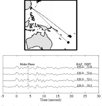
Figure 10. (a) Examples of radial-component receiver functions for TATO station showing similar receiver function waveforms for earthquakes from the southeast. (b) Inversion results for TATO-SE are shown with the same format as in Fig. 7. A mid-crust discontinuity can be identified at depth  $\sim$ 20 km which can be interpreted as the Conrad discontinuity. The preferred Moho depth is around 36 km.
