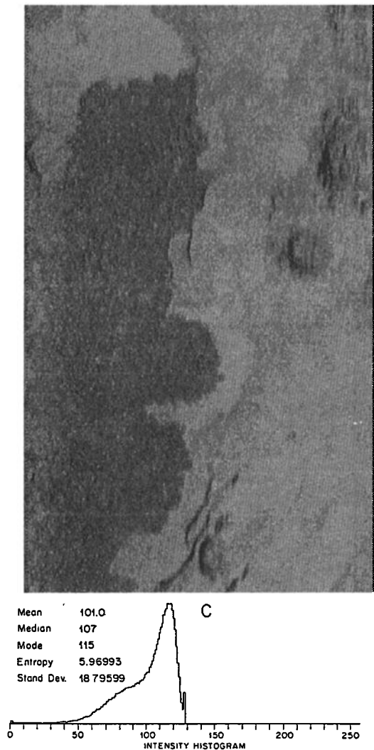
Figure 15c. The same image as shown in Figures 15a and 15b, but now subjected to a pixel amplitude “stretch” of 0.5 (dividing the pixel amplitudes by 2, which is actually a histogram compression). Again, the image becomes darker and much lower in contrast. These operations do not, obviously, improve the image and are shown as examples of specific histogram manipulations. Histogram equalization, which is a combination of sliding and stretching, is the operation normally done for image enhancement in the initial stages of processing.
