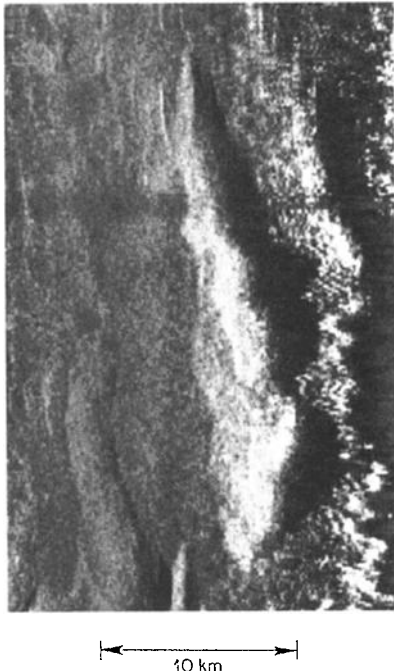
Figure 1. GLORIA image from the Washington margin, showing two anticlinal hills at 2000 m depth. Bright pixels are hard acoustic returns, and dark pixels are soft returns or acoustic shadows (the traditional GLORIA polarity). The bright pixels on the left flank of the hill on the right-hand portion of the image are returns due to proposed carbonate deposits associated with the dewatering of sediments during subduction. The anticlinal hill in the lower left of the image is of similar topographic relief but does not show comparable bright reflections. (Data from U.S. Geological Survey.)
