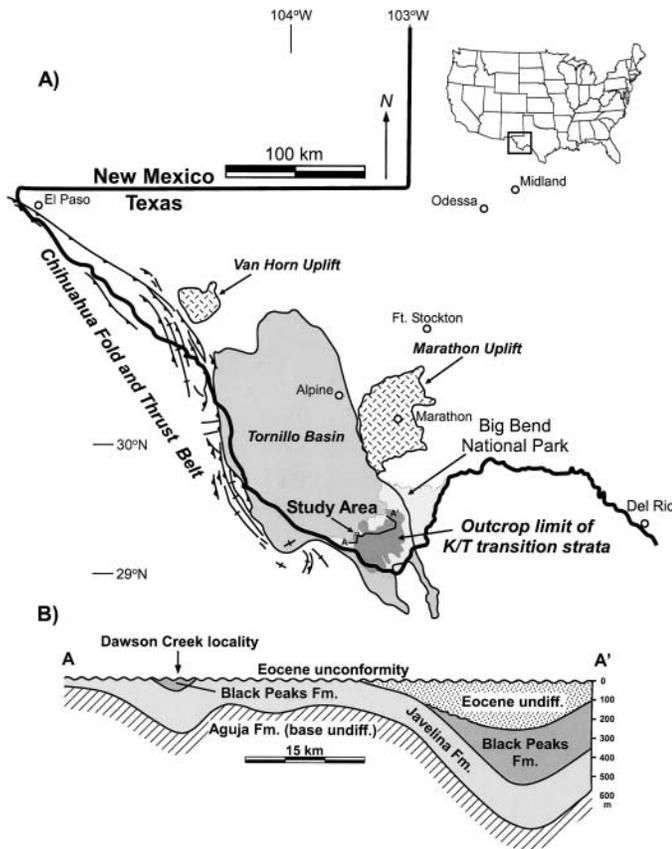
FIG. 1.—A) Map illustrating position of study area within the Tornillo Basin, and the distribution of other major Laramide structural features (modified from Lehman 1991). B) Diagrammatic cross section through the southeastern axis of the Tornillo Basin. Outcrop exposures along Dawson Creek are located approximately 50 km west of the basin axis (modified from Lehman 1986).
