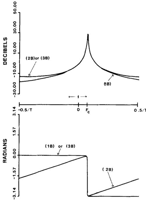
**Figure 1.** Transfer functions (1b) and (2b) displayed as amplitude in decibels ( $20 \log_{10}$  of the modulus of the transfer function) and phase (arc tangent of the ratio of imaginary to real parts). Calculations were done for the case  $T = 1$  month,  $F_c = 0.843$  cycle  $\text{yr}^{-1}$ , and  $Q_c = 100$ .
