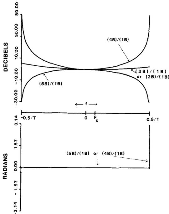
Figure 2. Transfer function ratio (4b)/(1b) and (5b)/(1b). The amplitude of the ratio is displayed in decibels. The phase of the ratio is the phase difference, which averages about  $3 \times 10^{-4}$  except near the Nyquist frequencies,  $\pm 0.5/T$ . The phase difference of (3b)/(1b) remains small even at the Nyquist frequencies.
