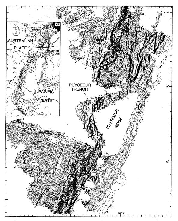
Figure 1. Multibeam bathymetric map of Puysegur Ridge and Trench; bathymetric contour interval is 50 m. Inset: Location of study area along Macquarie Ridge complex; NZ--New Zealand; Fi---Fiordland.
