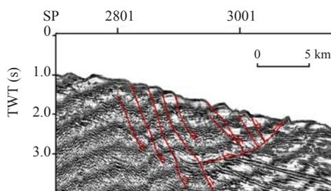
**Fig.8** Sea-dipping normal faults and thrusts formed by mass movement in the continental slope (See Fig.3 for position)
