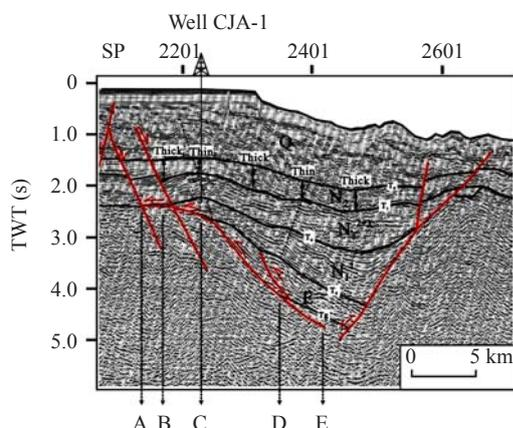
**Fig.4** Inverse structures in the faulted-sag (broken line represents the axis direction of the fold. A-B: fault flat; B-C: hanging wall fault ramp; C-D: lying wall fault ramp; D-E: fault flat)
