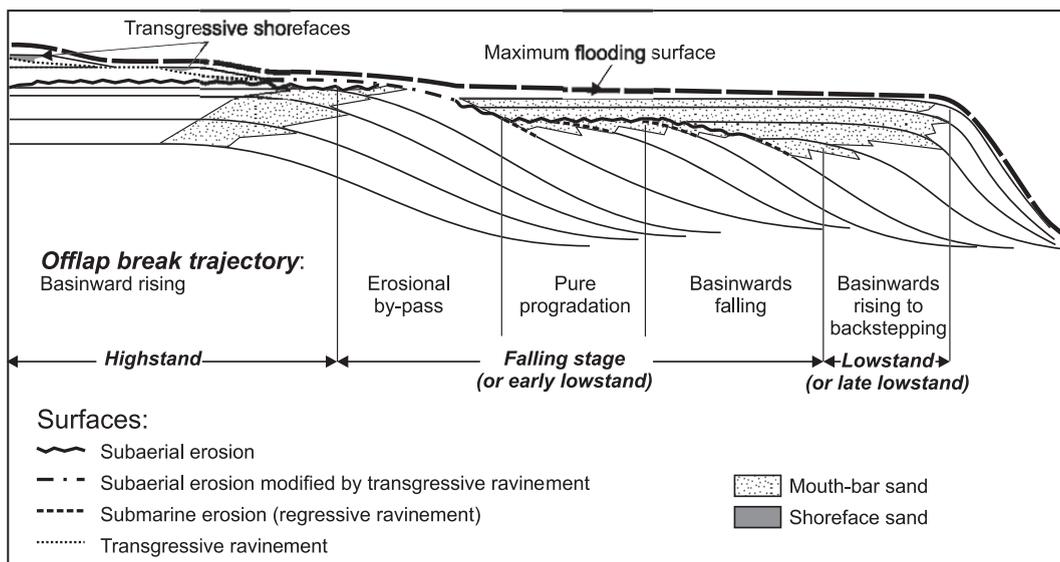
Fig. 11. Concept of offlap break trajectory (partly based on Helland-Hansen and Martinsen, 1996) and architectures of shelf-margin deltas.
