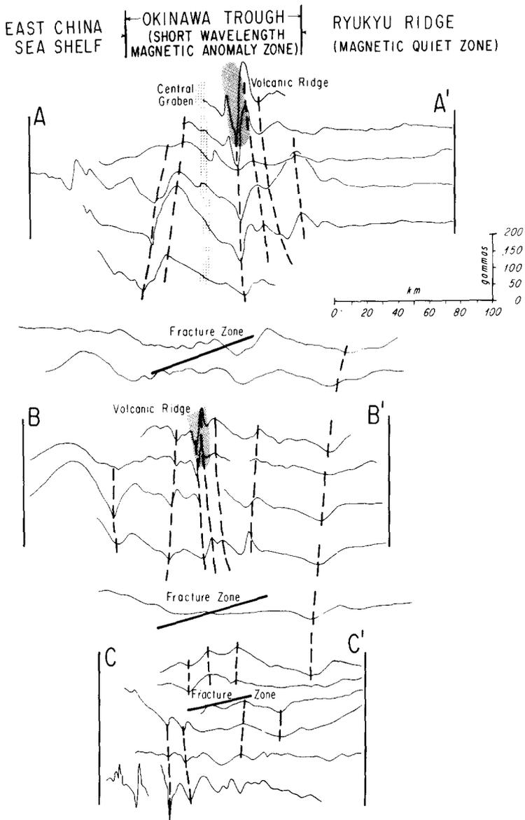
Fig. 4. Magnetic anomaly profiles across the southwestern Okinawa Trough projected onto an azimuth  $165^\circ$ . The heavy dashed lines indicate the lineations. The heavy solid lines represent suspected transform faults. Location of profiles A-A', B-B' and C-C' are shown in Fig. 3.
