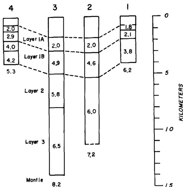
Fig. 6. Correlation of seismic refraction results in the Okinawa Trough. Data are taken from: 1 = Ludwig et al. (1973); 2 = Murauchi et al. (1968); and 3 = this study and 4 = Leyden et al. (1973).
