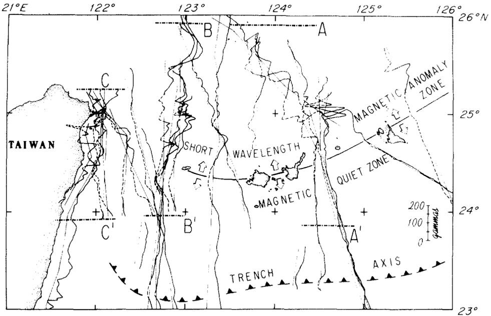
Fig.3. Magnetic anomalies in the southwestern Okinawa Trough and vicinity. Magnetic anomalies are plotted at right angles to the ship tracks. The heavy solid lines represent positive anomalies. The heavy dashed lines represent negative anomalies.
