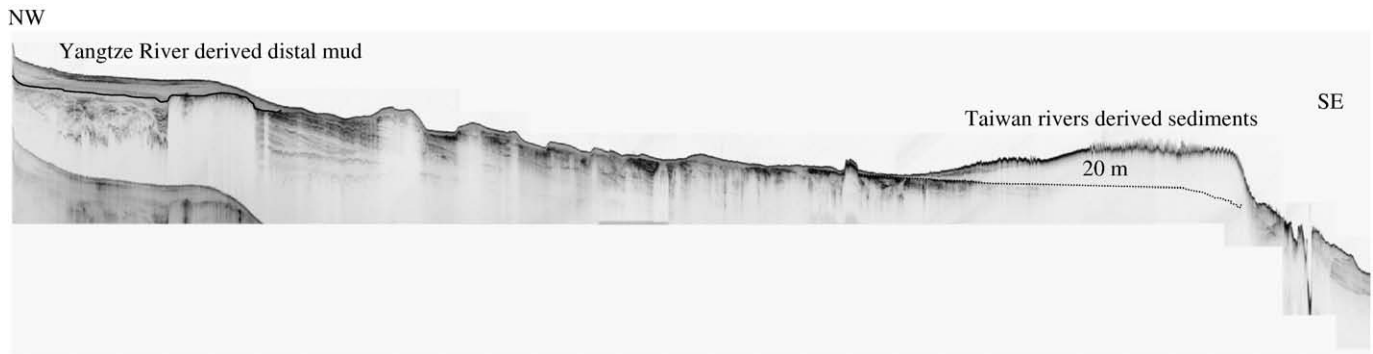
Fig. 10. Chirp sonar profile in the north Taiwan Strait, southern ECS, shows the Yangtze long-shore transported mud in the northwest, and possible Taiwan derived sediment in the middle shelf, north of the Taiwan island. See Fig. 4 for profile.
