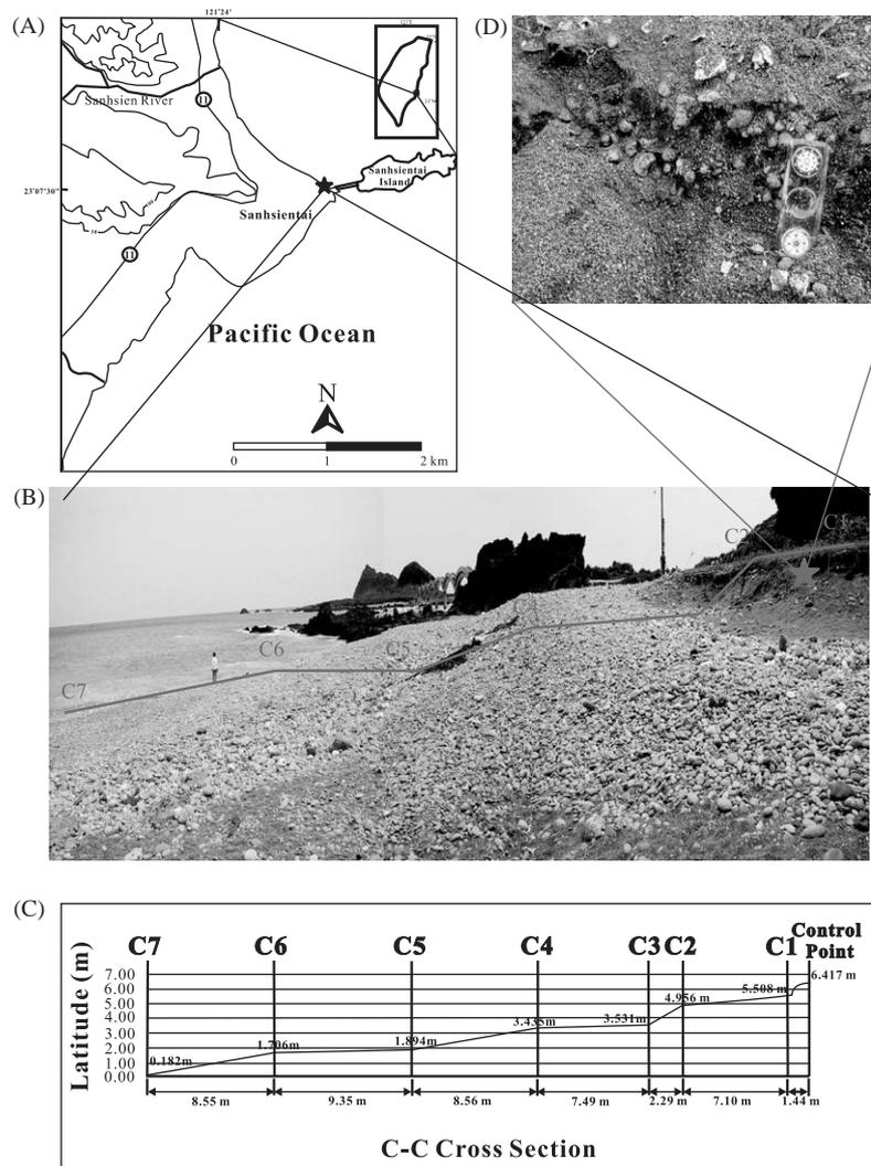
Fig. 2. (A) Map showing the location of the marine terrace in the Sanhsientai area, the southeast coast of Taiwan. (B) Photograph indicating the measuring points of latitude in the cross-section of the Sanhsientai marine terrace using the precise leveling method. (C) Results of latitude in the cross-section of the marine terrace in the Sanhsientai area. (D) Occurrence of the pumice-rich layer in the Sanhsientai marine terrace.
