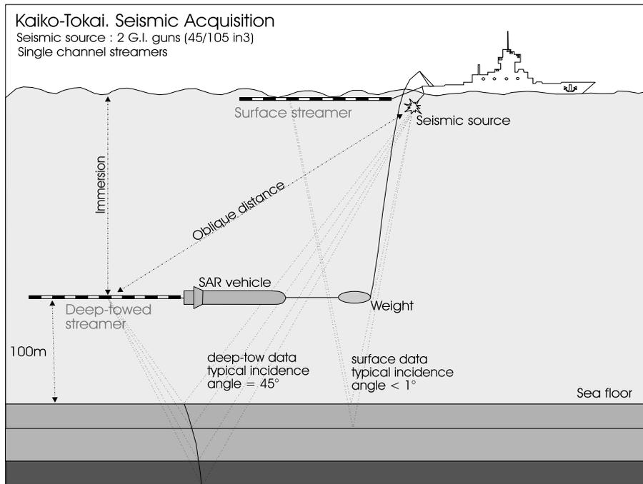
Fig. 2. Sketch illustrating the use of a deep-tow streamer (PASISAR towed at 100 m above seafloor) during the KAICO-Tokai cruise, in addition to a conventional surface streamer. Reflection points plot on a hyperbola, assuming horizontal reflectors and uniform velocity (1500 m/s) in water and sediments.
