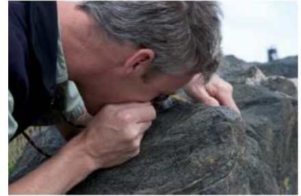
Figure 2.2 Photograph to show correct use of the hand lens. Note that the person is holding the lens close to his eye. The lens is fastened on a lanyard around his neck for ease of access and use.
