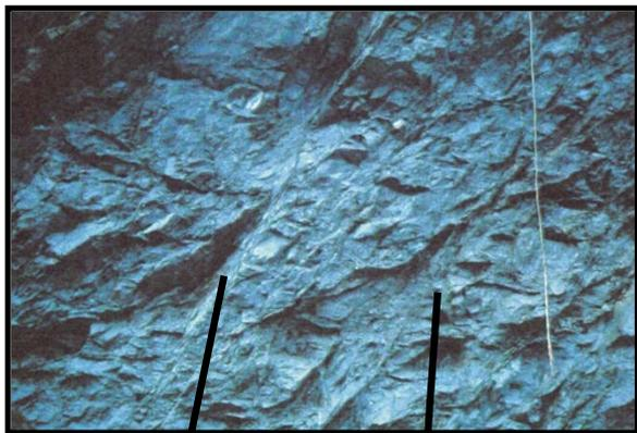
**Scaly foliation associated with shear deformation in the argillaceous matrix**
