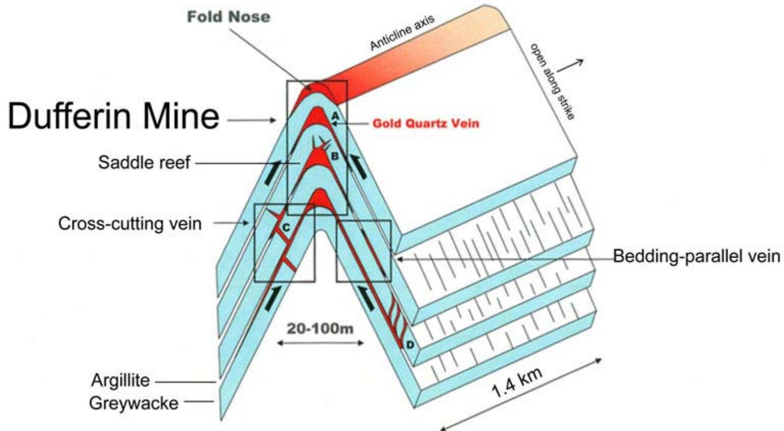
Schematic diagram for turbidite-hosted gold mineralization
