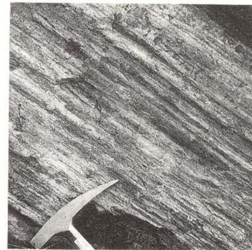
Fig. 5.6d Grooving on a fault plane in limestones.
