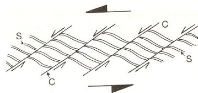
Fig. 6.26a The geometry of C and S fabrics as seen in shear zones. The C plane is the shear plane and S is the schistosity plane. The C plane has an extensional geometry with respect to the sense of shear. (Fig. 6.26b on p. 112)
