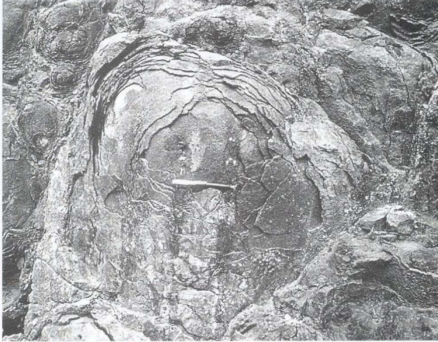
Fig. 1.2 Spheroidal weathering in granite. Note low successive, thin layers of weathered rock are spalled off to produce a spheroidal core.
