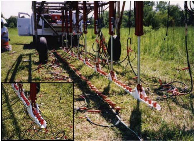
Figure 1. Photograph of the coincident CMP data-acquisition geometry. The Autojuggie II uses hydraulic cylinders to lower and raise the channel-iron segments to which the test-line geophones (right line) are attached. Two cylinders work in tandem on each segment. Eighteen geophones are attached to each piece of channel iron at 12-cm intervals. All 72 geophones were planted in approximately 90 s. The channel-iron segments can be raised \sim 1 m above the ground for transport. The inset shows the cylinders in the raised position and the configuration of the geophone and the spike on the channel iron.
