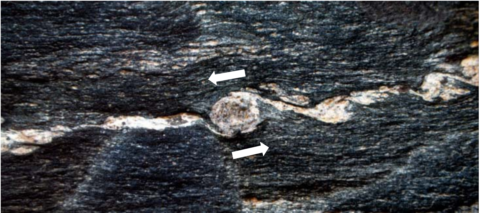
Figure 15.29 \delta -porphyroclast indicating rotation during top-to-the-left shearing, consistent with the asymmetry of small-scale folds (right).
