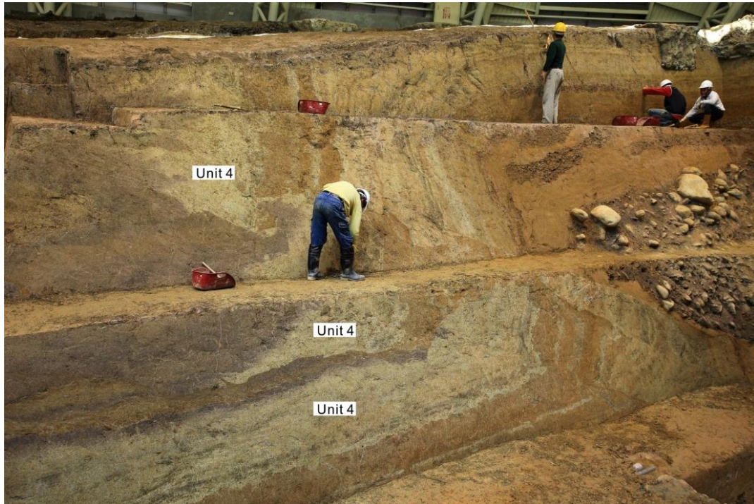
Fig. 5-56. Structures exposed in the north wall of Chushan trench excavated in 2012. The difference of structures on the north walls in between 2012 and 2002 (Fig. 5-54A) is observable, in particular, via Unit 4. Unit 4: bluish sandy, clayey silt. [Photograph by Liu Yung-Chu]
