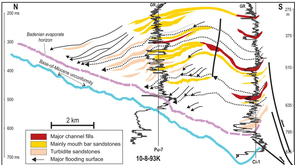
Fig. 8. Interpreted line drawing from seismic dip-section through Badenian shelf margin in the Carpathian foredeep (southeast Poland), showing the distribution of sand bodies (Porębski et al., in press). Note that the sand bodies thin and pinch out landwards (to the south), and form the thickest accumulation near the shelf edge which is constructed mainly of mouth-bar and slope turbidite sandstones. See Fig. 19B, for location of section.
