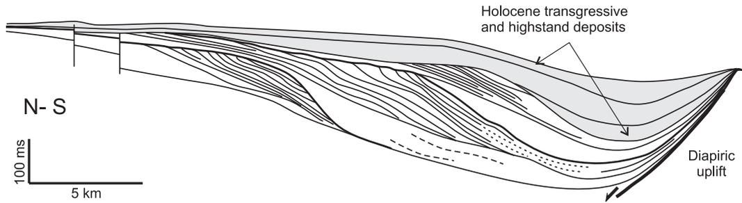
Fig. 24. Minisparker seismic section through late Wisconsinan Mississippi delta, showing the progradation and aggradation of deltaic shelf edge due to relative sea-level rise generated by local, diapir-related subsidence (after Suter and Berryhill, 1985).
