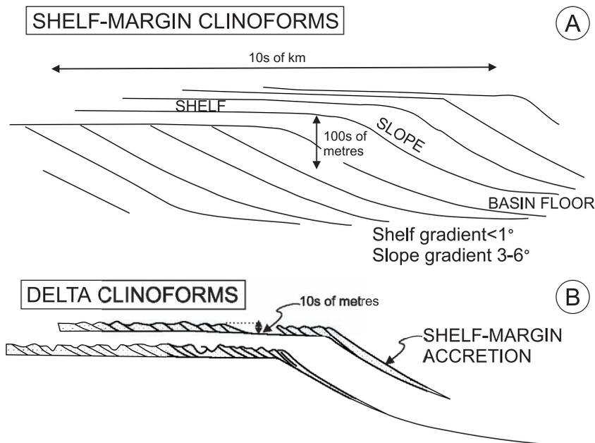
Fig. 3. Distinction between clinoforms generated by (A) shelf-margin accretion, and by (B) prograding shelf deltas. Note that the two types coincide only when deltas reach the shelf edge and drape partly down the slope.
