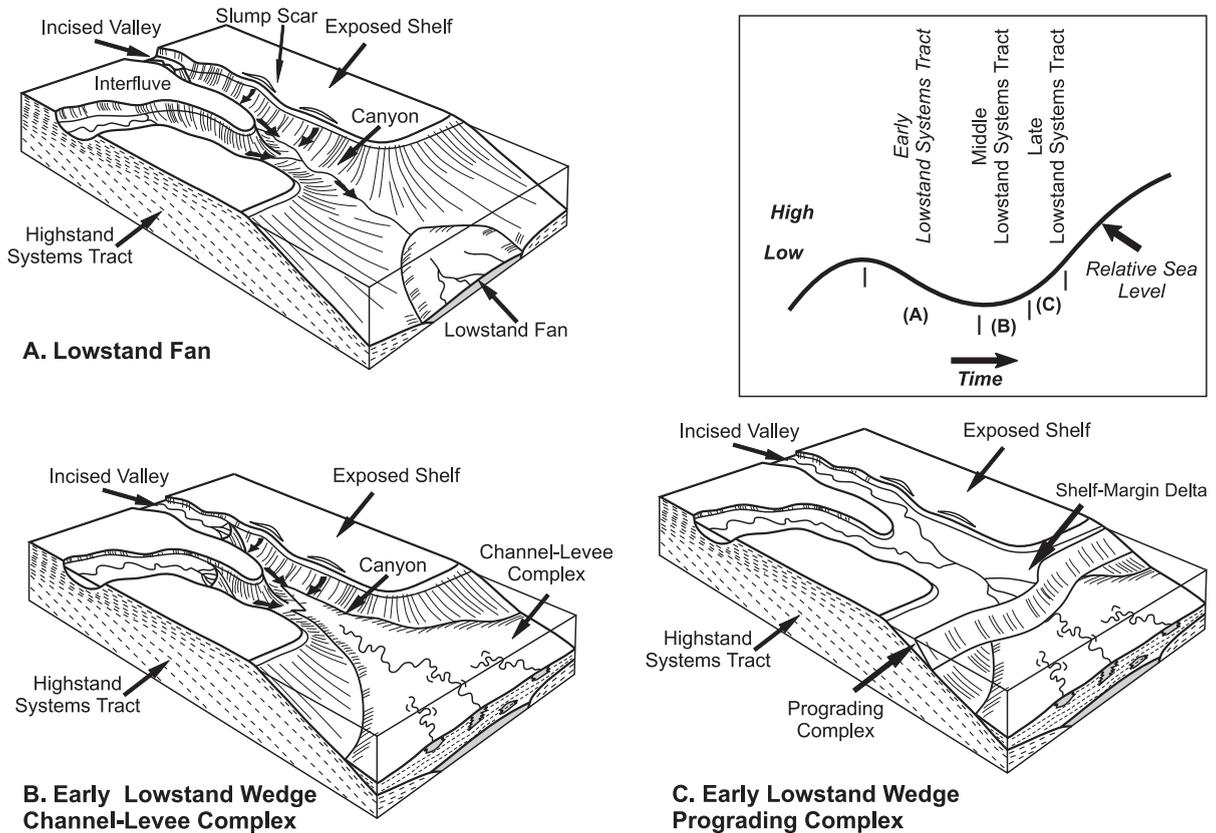
Fig. 25. Block diagrams of the lowstand systems tracts (modified from Posamentier et al., 1991; Normark et al., 1993). Note that the deposition of basin-floor fan is promoted when incised valley becomes linked to canyon on the slope during relative sea-level fall (A), while shelf-margin delta is the dominant component of the prograding complex that is formed during early rise (C).
