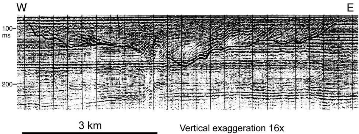
Fig. 22. Transverse seismic section through Late Pleistocene fluvial channel in outer Louisiana shelf, showing compound infill (after Suter and Berryhill, 1985).
