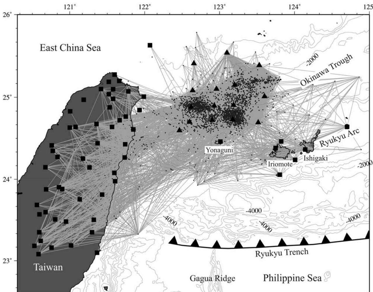
**Figure 3.** The 2-D  $P$  wave ray coverage shown by gray lines between earthquakes (dark gray dots) and seismic recording stations. The OBS (black triangles) recorded earthquakes during a period of 12 days (3353 events). Black squares are the locations of seismic land stations of the Central Weather Bureau and Japan Meteorological Agency networks. Bathymetric contours are every 500 m.
